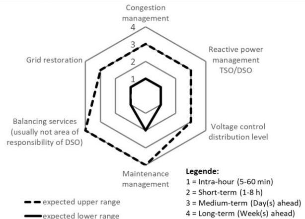
Figure 1: Expected relevant PV forecasting horizons for different applications in distribution network operation. For the multi-use case storage, the requirements dependent on the selected use cases.
