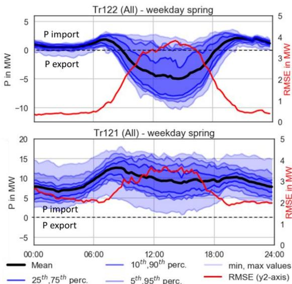
Figure 3: Statistic evaluation of active power transfer at HV/MV transformer Tr122 (top) and Tr121 (bottom) for all spring weekdays in 2017
